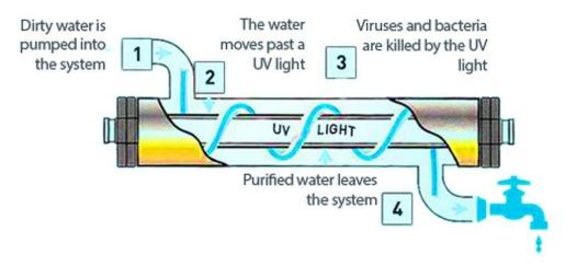
The glass quartz sleeve holds the UV lamp and protects it from direct contact with the water. It is transparent to the UV wavelength, which allows UV light to penetrate the glass and disinfect the water. A couple of O-rings hold it in place and prevent leakage.
